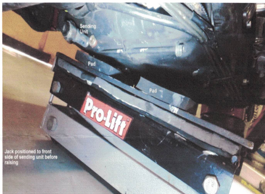
Note: Adapter positioned to avoid sending unit
