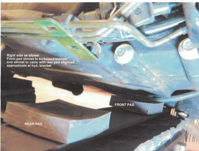
Note: Pad positioned to front of bike motor With rear aligned to avoid sending unit front pads Will be in this approximate position with adapter Rolled just to cable and kickstand bracket.
